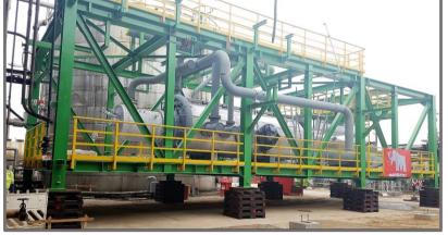
Sulfur Recovery Units: Thermal Oxidizers
