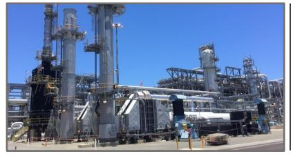
LNG Liquefaction Thermal Oxidizers
